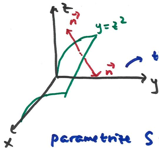
this is the one with component in pos.  $y$ -axis direction
