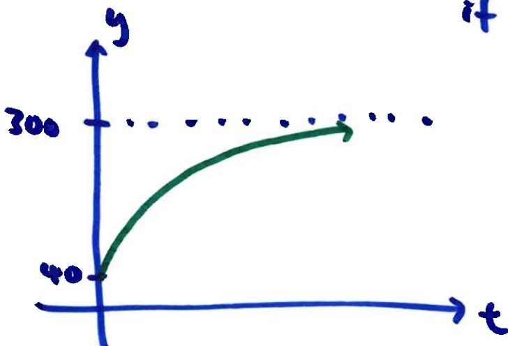
after a while, the tank is like a pipe because rate in = rate out
