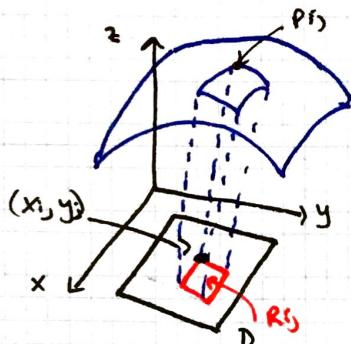
We want to compute the area of a surface  $z = f(x, y)$  above a rectangle  $D$ . We'll assume  $f(x, y) \geq 0$  on  $D$ . We'll approximate the area  $\Delta S_{ij}$  of a patch lying above the rectangle  $R_{ij}$  by the area  $\Delta T_{ij}$  of the tangent plane lying directly above  $S_{ij}$ . If  $\vec{a}, \vec{b}$  are the vectors starting at  $P_{ij}$  along the sides of the parallelogram  $T_{ij}$ , then  $\Delta T_{ij} = |\vec{a} \times \vec{b}|$ .
