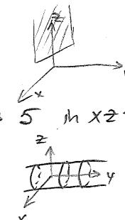
(b) cylinder whose base is a circle of radius 5 in  $xz$ -plane centered at the origin and with axis along the y-axis
