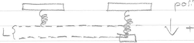
By Hooke's Law, the spring force is proportional to the length  $L$  that the mass stretches the spring.
