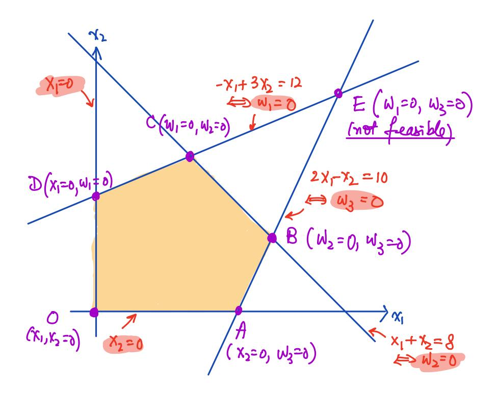
(0) max  $\int = 3x_1 + 2x_2$ Subject to  $W_1 = 12 + \chi_1 - 3\chi_2$  $W_2 = 8 - \chi_1 - \chi_2$  $\omega_3 = 10 - 2\kappa_1 + \kappa_2$  $\chi_1, \chi_2, \chi_3, W_1, W_2, W_3 \ge 0$ X1, X2, X3 on the RHS - non-basic variables W, W2, W3 on the LHS - basic variable Idea of Simplex Mothod: (1) set all non-basic var. to zero - correspond to a vertex (2) choose a new set of (non) basic vars, to improve f. ((1) of (2) is the same as moving from vertex to vertex.)
